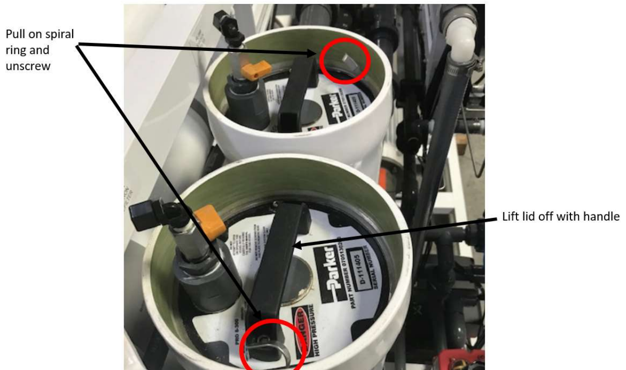
Figure 7.2 – Filter Change Out
